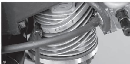
1. Put a lock washer on each of the muffer screws. Push the muffer screws through the cylinder head.
