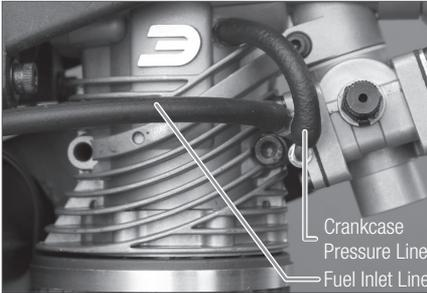
1. Connect medium diameter tubing to the carburetor and the fuel tank supply line.
