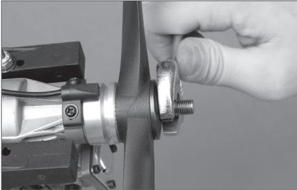
1. Remove the prop nut and prop washer from the crankshaft.
